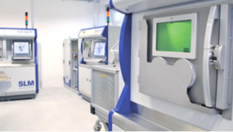
Our additive manufacturing method is based on SLM-Technology (short for **selective laser melting**). It is a beam melting procedure and is commonly known as 3D printing of metal.
